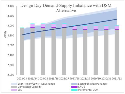
Figure 8-3: Design Day Demand-Supply Imbalance with DSM Alternative
